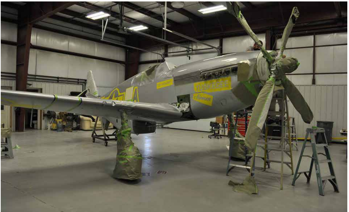
Plotter cut spray mask applied to various areas of the aircraft as part of the traditional Tuskegee graphics package Follow our Facebook page for the latest updates!
